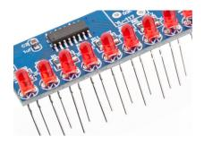
When all the surface mounted components are in place, continue with the LEDs, the potentiometer and the pin header. All the LEDs should be facing the same direction. The short leads should be inserted in the holes closest to the 8-pin IC. You can also refer to the symbols on the PCB.
