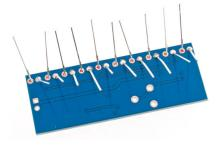
Flip the board and notice the poor alignment. Melt the solder and press down on each LED to align them properly. When they are all in a straight line, solder the other lead.
