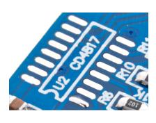
Place and align the IC using tweezers. Make sure both rows of the IC align up with the pads. Alignment must be correct
