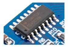
Continue soldering the rest of the pins. If you should bridge two pins with solder, you have a few options. You can melt the solder and quickly drag the tip away from the IC to break the bridge. If this doesn't work, try adding flux. A last resort is to use a desoldering pump to remove the excessive solder.
