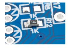
Solder the opposing pad. Redo the first pad if necessary. Continue mounting the rest of the passives.
