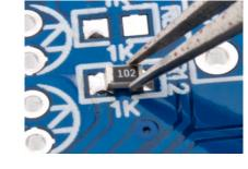
Place the component on the correct place on the board. Use tweezers to hold the component (unless you have really tiny, heat-resistant fingers).
