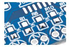
Start by pre-tinning one pad for each of the passive components. Only a small amount of solder is required.
